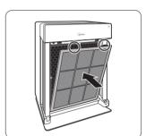
③ Replace the front panel by first inserting the latch at the bottom edge into the base of the unit, then rotate the panel upward toward the top of the unit until it magnetically snaps closed.
