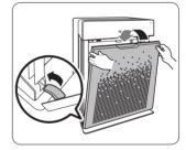
4 After replacing the filters, turn the power back on and then use a thin object, such as a paper clip, to press the RESET switch for 5 seconds.
