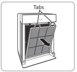
③ First remove the 2 AOC™ Carbon Filter and then the 3, 4 True HEPA filter with Cleancel™ by pulling on the numbered tags at the top of each filter.
