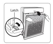
② Press the tabs on the top edge to remove the 1 Pre-filter.
