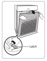
② Remove the filters from the unit, they are protected inside a plastic wrap.
